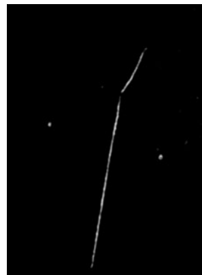
The nuclear reaction n + {}^{14}\text{N} \rightarrow {}^{11}\text{B} + \alpha as observed by Feather in a cloud chamber. The neutron (leaving no track) enters from the left and reacts with a nitrogen nucleus of the chamber gas. The short track is due to the boron nucleus, the long one to the \alpha particle. From [9], Fig. 18. Reprinted with permission.
