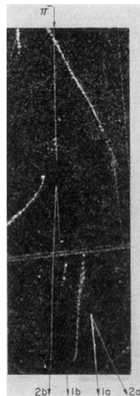
Early observation of associated production in a cloud chamber. The photograph (one of a stereoscopic pair) shows the stopping of the track of an incoming \pi^- meson. Only neutral particles are produced in the interaction of the pion with a proton. Two neutral particles are seen to decay into pairs of charged ones, a \Lambda^0 into a proton (track 1a) and a \pi^- (2a), and a K^0 into a \pi^+ (1b) and a \pi^- (2b). Figure reprinted with permission from [8]. Copyright 1954 by the American Physical Society.
