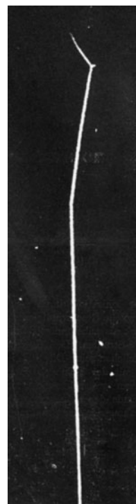
An \alpha particle, coming from below, is scattered twice by nuclei from the gas filling of the chamber. The recoil nucleus of the second scattering itself leaves a track. From [3], Plate 6.3. Reprinted with permission.
