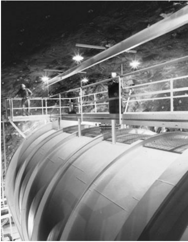
The chlorine detector of Davis in the Homestake Gold Mine. Photo: Brookhaven National Laboratory.
