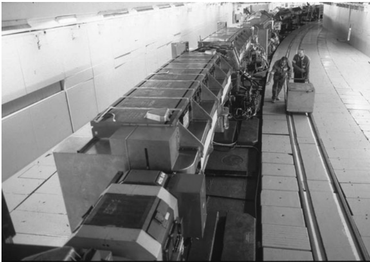
Section of the 25-GeV CERN Proton Synchrotron. Designed as an alternating-gradient machine, the total iron weight of its magnets is 3400 tons, only about a third of the weight of the Bevatron magnets, while it reaches four times the Bevatron energy. Photo CERN.
