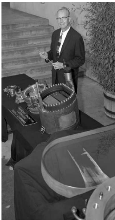
Alvarez with various bubble chambers built in his group. In front the glass window of the 72-inch chamber.
