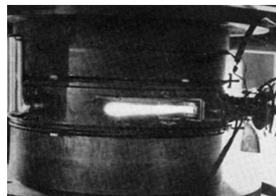
A deuteron beam, in air, produced by the 37-inch cyclotron. Figure reprinted with permission from [11]. Copyright 1936 by the American Physical Society.
